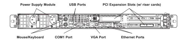
**Note:** the SC815TQ-560U chassis (6015W-U/6015W-NT) has only a single power supply module.
